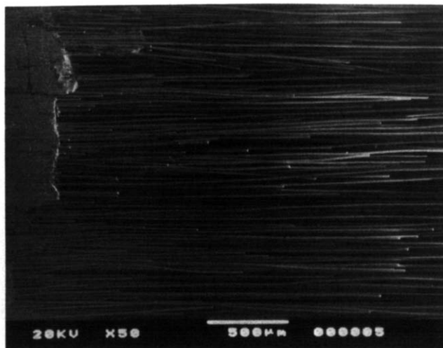
Fig. 11. SEM micrograph showing long pull-out lengths in these unidirectional SiC-MAS.L composites.
